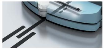
The MLS reliably differentiates up to three magnetic lines. In addition, positions or commands (such as for turning at intersections) can be coded using lateral magnet marks.
