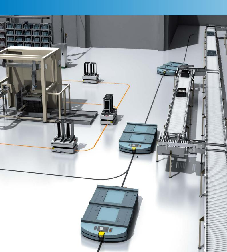
Autonomous material transport systems are now used in nearly every single area of the production industry. Whether you use automated guided vehicle systems, semi-automated guided vehicle systems, transfer cars, manned forklift trucks, or narrow aisle trucks – a whole host of different sensor functions has to be performed – such as for navigation, as well as for rough and fine positioning of vehicles, transporting the load or for protection of people, the load and the vehicle.
