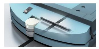
The MLS is mounted at a 90° angle to the magnetic line. Thanks to different variants with a detection range of 200 mm to 600 mm, there is an appropriate solution for every vehicle.
